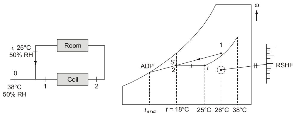
Draw RSHF line, its intersection with  $t = 18^\circ\text{C}$  vertical given supply air state point s-which is the same as coil leaving air state point-2.
