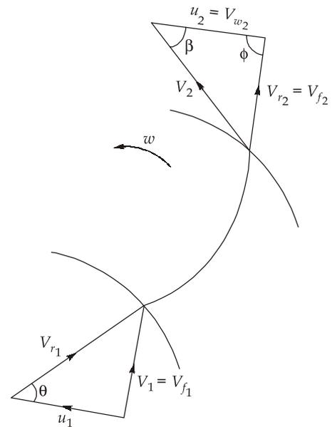
$$\eta_{\text{manometric}} = \frac{H_m}{\frac{V_{w2} u_2}{g}}$$
