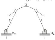
**Note:** The degree of freedom of given figure is 1, but still it is structure.
