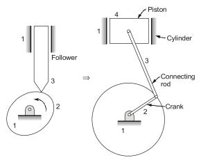
Here H.P. between link 2 and 3 is replaced by 2 L.P. (revolute pair) with one additional linkage.
