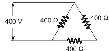
$$I_{Ph} = \frac{V_{Ph}}{R_{Ph}} = \frac{400}{400} = 1 \text{ A}$$
