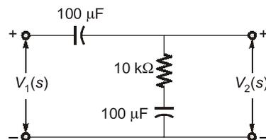
$$\frac{V_2(s)}{V_1(s)} = \frac{R + \frac{1}{Cs}}{\frac{1}{Cs} + R + \frac{1}{Cs}} = \frac{1 + RCs}{2 + RCs}$$
