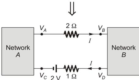
$$\begin{aligned} \Rightarrow V_A - V_B &= 2I \\ \Rightarrow 2I &= 6 \\ \Rightarrow I &= 3 \text{ A} \\ V_C + 2 + 1 \times I &= V_D \\ V_C - V_D &= -2 - 3 \\ &= -5 \text{ V} \end{aligned}$$
