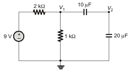
By applying voltage divider rule.
