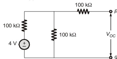
$$V_{OC} = 4 \times \frac{100}{100 + 100} = 2 \text{ V}$$
