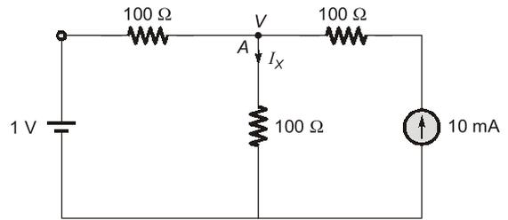
Applying Node equation at Node A
