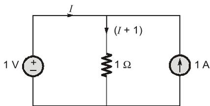
By applying KVL in 1<sup>st</sup> loop
