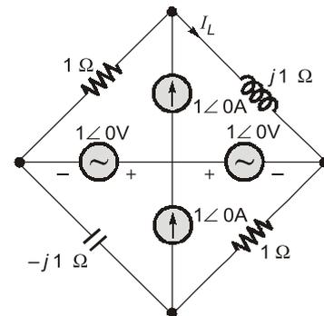
By applying current division rule in upper part of the circuit.
