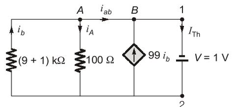
To find Thevenin impedance across node 1 and 2. Connect a 1 V source and find the current through voltage source.
