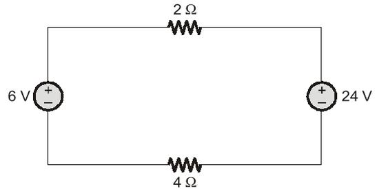
$$I = \frac{V_2 - V_1}{6} = \frac{24 - 6}{6} = 3 \text{ A}$$
