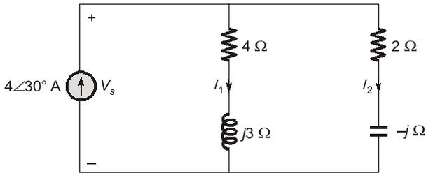
$$\begin{aligned} V_S &= I_1(4 + 3j) \\ &= (1.414 \angle -15^\circ)(4 + j3) \\ &= 7.07 \angle 21.87^\circ \text{ V} \end{aligned}$$
