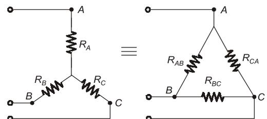
$$R_{AB} = R_A + R_B + \frac{R_A R_B}{R_C}$$
