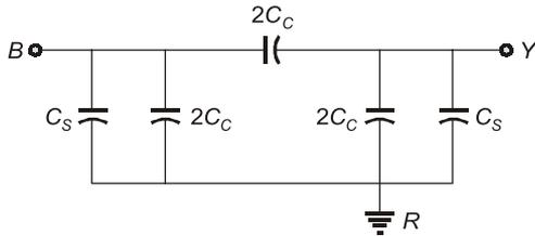
$$C_{BY} = \frac{C_s + 2C_c}{2} + 2C_c = \frac{C_s + 6C_c}{2}$$
