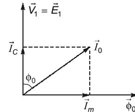
Here, no load current ( $I_0$ ) cannot lag  $\vec{V}_1$  by  $90^\circ$  because of core loss. In practical transformer,
