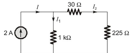
$$I_2 = 2 \times \frac{1\text{k}\Omega}{1\text{k}\Omega + 225 + 30} = 1.59 \text{ A}$$
