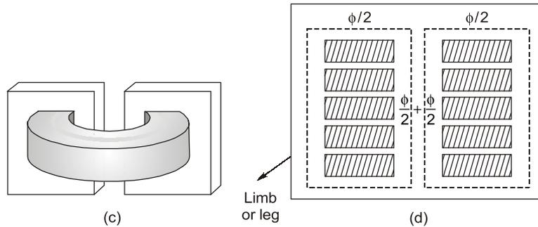
**Fig. : Constructive Details of Shell Type**
