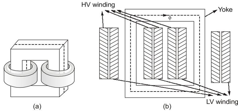
**Fig. : Constructive Details of Core Type**
