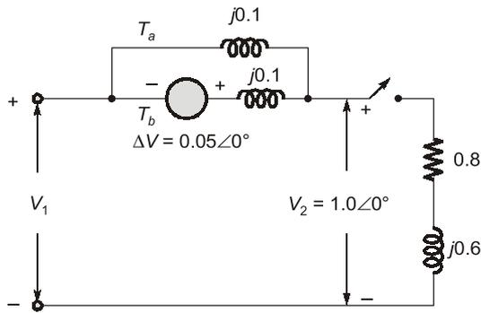
Transformer  $T_a$  has a voltage ratio equal to the ratio of the base voltages on the two sides of the transformer. This transformer has an impedance of  $j0.1$  p.u. on the appropriate base. The second transformer  $T_b$  also has an impedance of  $j0.1$  p.u. on the same base but has a step up toward the load of 1.05 times that of  $T_a$  (secondary windings on 1.05 tap). Figure shows transformer  $T_b$  represented by its impedance and the insertion of the voltage  $\Delta V$ .
