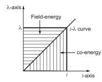
Where,  $\lambda = N\phi = Flux linkage$
