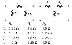
**Q.5** For the equivalent figure circuit shown in the given figure, the values of  $R_{AB}$  and  $R_{BC}$  are respectively
