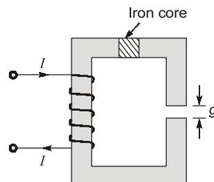
Calculate and compare the field-energy stored and field-energy density in iron as well as in airgap. Neglect fringing and leakage flux.
