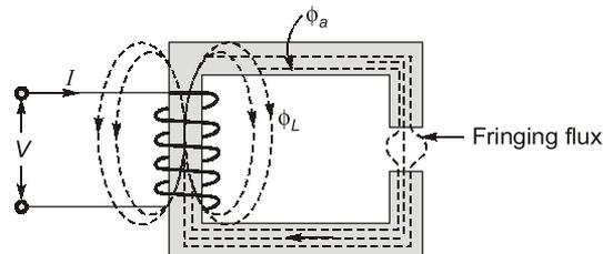
Of the total flux generated by the coil, some flux  $\phi_L$  does not follow the intended path of the magnetic circuit. This flux cannot be used for any purpose. This flux is called as the leakage flux.
