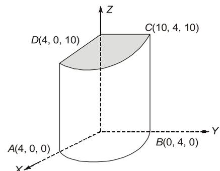
**Q.27** If  $\vec{A} = \hat{a}_\rho + \hat{a}_\phi + \hat{a}_z$ , the value of  $\oint \vec{A} \cdot d\vec{l}$  around the closed circular quadrant shown in the given figure is \_\_\_\_\_.
