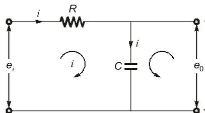
(b) Find the transfer function of circuit shown below.
