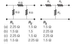
**Q.5** For the equivalent @ figure circuit shown in the given figure, the values of  $R_{AB}$  and  $R_{BC}$  are respectively
