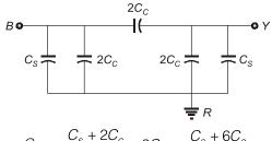
$$C_{BY} = \frac{C_s + 2C_c}{2} + 2C_c = \frac{C_s + 6C_c}{2}$$
