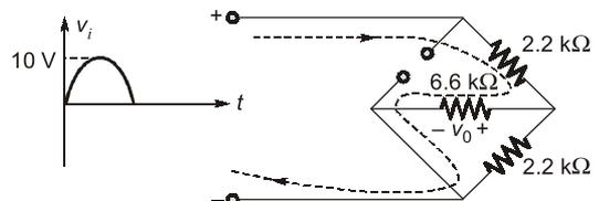
$$V_{O_{max}} = \frac{[6.6 \text{ k}\Omega \parallel 2.2 \text{ k}\Omega]}{2.2 \text{ k}\Omega + [6.6 \text{ k}\Omega \parallel 2.2 \text{ k}\Omega]} V_{i_{max}}$$
