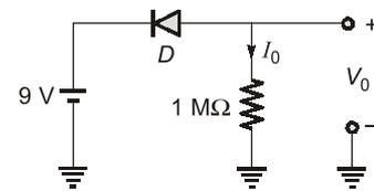
The diode in the circuit is a large high-current silicon device whose reverse leakage current is reasonably independent of voltage appearing on the diode. If  $V_o = 1 \text{ V}$  at  $20^\circ \text{C}$ , then the value of output voltage at  $40^\circ \text{C}$  is equal to \_\_\_\_\_ V.
