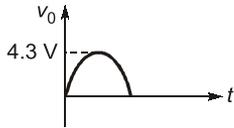
For negative half cycle of input voltage
