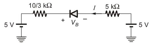
Applying KVL we get  $V_D = 0 \text{ V}$ , thus no current will flow through the diode  $D_1$ .
