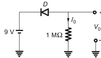
Calculating the value of reverse saturation current ( $I_{01}$ ) flowing through the diode at  $20^\circ\text{C}$
