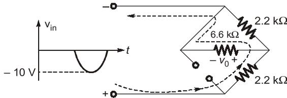
$$V_{O_{max}} = \frac{[6.6 \text{ k}\Omega \parallel 2.2 \text{ k}\Omega]}{2.2 \text{ k}\Omega + [6.6 \text{ k}\Omega \parallel 2.2 \text{ k}\Omega]} V_{i_{max}}$$
