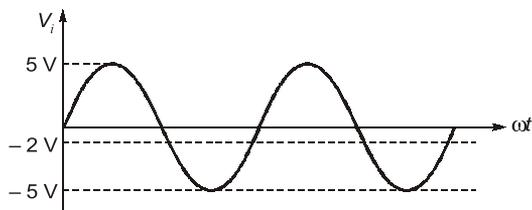
Hence given circuit acts as a clamper, sine wave clamped at  $-2 \text{ V}$ .
