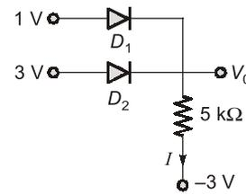
If diode  $D_1$  and  $D_2$  are made up of same material with the cut-in voltage  $V_\gamma = 0.7 \text{ V}$ , then the value of current  $I$  is equal to
