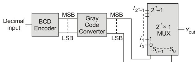
If the decimal input is 92 then  $Y_{\text{out}}$  corresponds to  $I_m$ , then value of  $m$  is \_\_\_\_\_.
