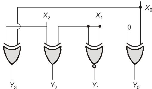
If the three bit input to the circuit is  $(X_2 X_1 X_0) = 111$  then the decimal equivalent of the
