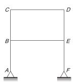
If the axial and shear deformations in different members of the frame are assumed to be negligible, then what would be the reduction in the kinematic indeterminacy.
