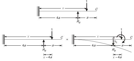
Deflection at B due to unit load at x is same as the deflection at x due to point load at B.
