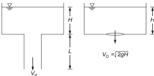
Reservoir with a long vertical pipe of length  $L$
