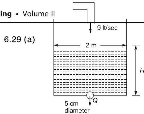
For steady level in the tank discharge released from the tank is equal to the water enter in the tank.
