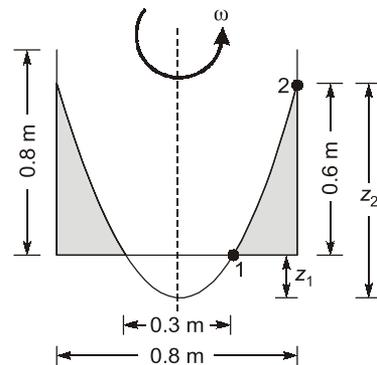
$$z_2 - z_1 = \frac{\omega^2}{2g} [R_2^2 - R_1^2]$$
