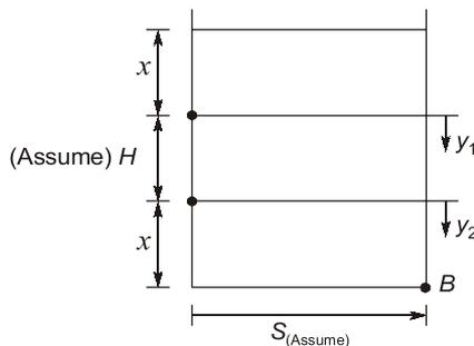
Assume  $C_v$  is same for both the orifice and the horizontal distance travelled by both the jets is same ( $S$ ).
