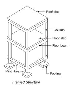
All the above elements of the frame are constructed monolithically. Framed structure is subjected to a variety of external loads like compressive, tensile, torsion and shear along with moment. R.C.C. is the most suitable material to withstand all these loads. Bricks can withstand only compressive loads, so all framed structures are constructed with R.C.C.
