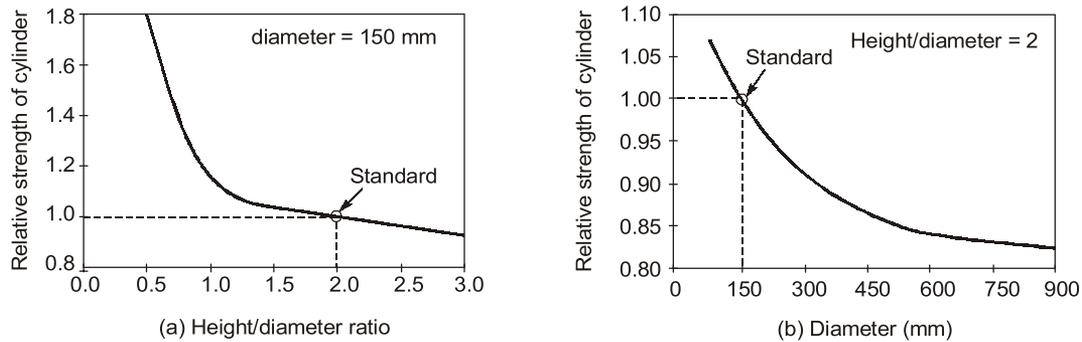
**Fig. :** Influence of (a) height/diameter ratio and (b) diameter on cylinder strength
