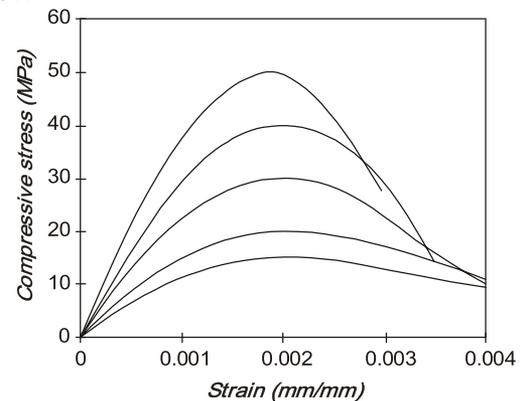
**Fig. :** Typical stress-strain curves of concrete in compression
