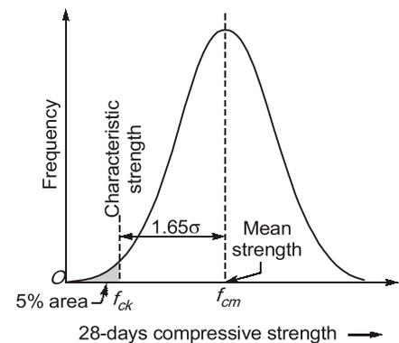
*Fig. : Idealised normal distribution of concrete strength*
