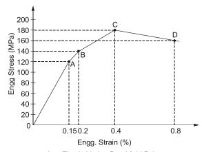
A → Elastic Limit; B → Yield Point  $C \rightarrow UTS$  Point;  $D \rightarrow Fracture$  Point
