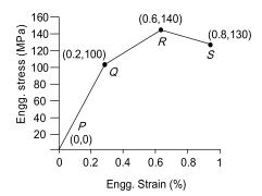
The toughness of the material (in MJ/m<sup>3</sup>) is\_\_\_\_\_.
