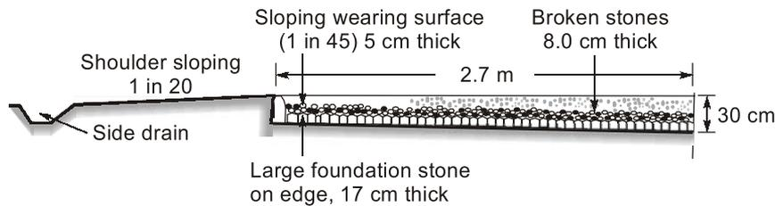
**Typical cross-section of Tresaguet's construction**
