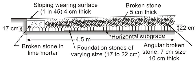
**Typical cross-section of Telford's construction**
