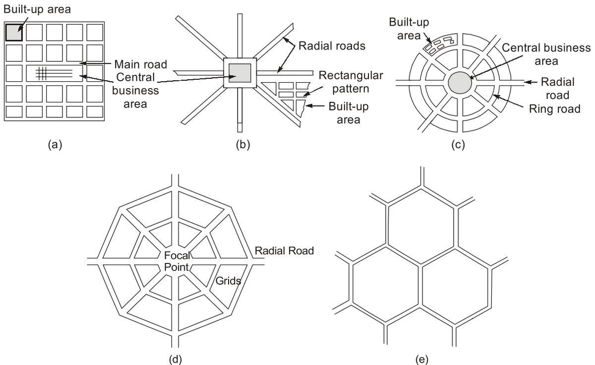
(a) Rectangular or Block pattern (b) Radial or Star and Block pattern
