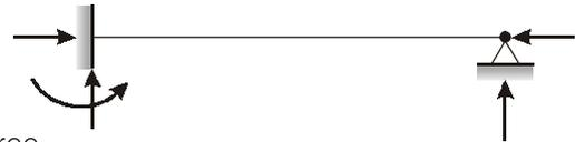
Hence given beam is externally indeterminate to 2<sup>nd</sup> degree.
