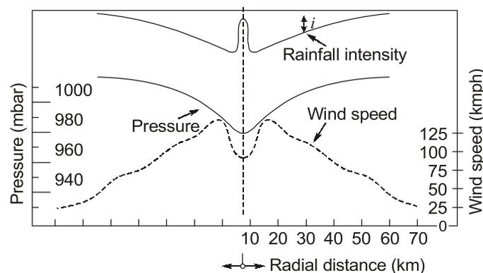
**Schematic Section of a Tropical Cyclone**
