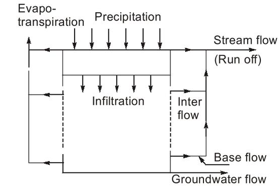
**Transportation Components of the Hydrologic Cycle**
