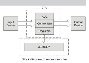
The figures shows the basic block diagram of a microcomputer which processes binary data and traditionally represented by four blocks i.e. CPU, memory, input device and output device.
