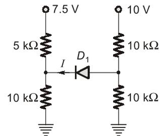
If the cut-in voltage of the diode  $D_1$  is equal to  $0.7 \text{ V}$ , then the value of current flowing through the diode is equal to \_\_\_\_\_ mA.
