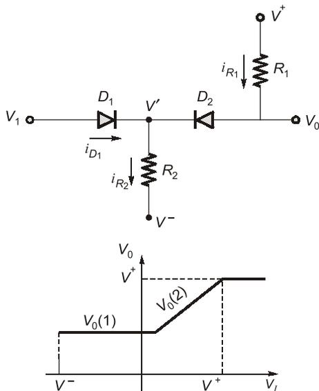
Assume the circuit parameters are  $R_1 = 5 \text{ k}\Omega$ ,  $R_2 = 10 \text{ k}\Omega$ ,  $V_\gamma = 0.7 \text{ V}$ ,  $V^+ = +5 \text{ V}$  and  $V^- = -5 \text{ V}$
