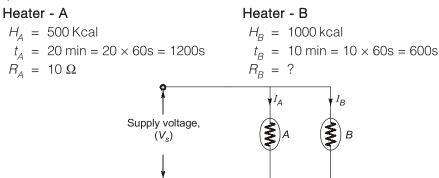
Consider the circuit shown above having current through heater A and heater B are  $I_A$  and  $I_B$  respectively. For a parallel connected heater,
