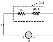
Case-2: When coil is connected to 65 V, 50 Hz ac supply frequency, f = 50 Hz
