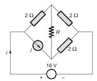
The given circuit is a Wheatstone's bridge. So, the current source I can be replaced by 2  $\Omega$ .
