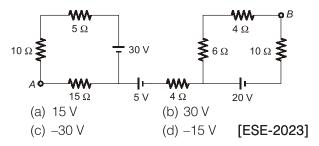
**1.87** What is the value of voltage at node  $V_A$  shown in the network below?
