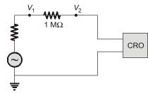
If  $V_1 = 5$  V and  $V_2 = 3$  V, then what is the input impedance of the CRO in the above circuit?
