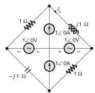
By applying current division rule in upper part of the circuit.
