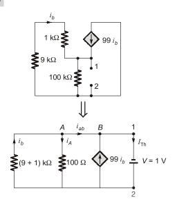
To find Thevenin impedance across node 1 and 2. Connect a 1 V source and find the current through voltage source.
