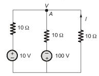
Let *V* is the voltage at node *A*. By applying KCL at node *A*
