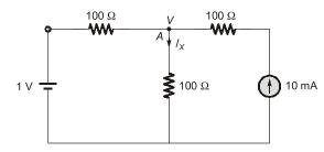
Applying Node equation at Node A
