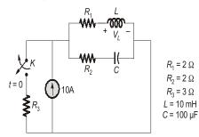
For time t < 0, the circuit is at steady state with the switch 'K' in closed condition. If the switch is opened at t = 0, the value of the voltage across the inductor ( $V_L$ ) at  $t = 0^+$  in Volts is \_\_\_\_\_ (Round off to 1 decimal place).
