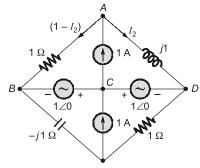
Apply KCL node at 'A', so, current flowing through 1  $\Omega$  is (1 –  $I_2$ )
