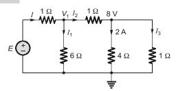
Voltage across 4  $\Omega$  resistor = 4  $\times$  2 = 8 V Current through 1  $\Omega$  resistor,
