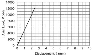
Assume the yield stress of steel as 250 MPa. The complementary strain energy (in N-mm) stored in the bar up to its linear elastic behaviour will be
