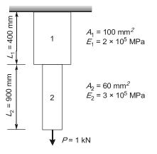
Segments 1 and 2 have cross-sectional area of 100 mm<sup>2</sup> and 60 mm<sup>2</sup>. Young's modulus of  $2 \times 10^5$  MPa and  $3 \times 10^5$  MPa, and length of 400 mm and 900 mm, respectively. The strain energy (in N-mm upto one decimal place) in the bar due to the axial load is \_\_\_\_\_.
