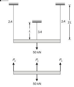
From symmetry, the force in each of outer rods is  $P_0$  and force in the central rod is  $P_C$ , then,
