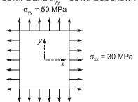
The Young's modulus of the material is  $2 \times 10^{11} \text{ N/m}^2$  and the Poisson's ratio is 0.3. If  $\sigma_{zz}$  is negligibly small and assumed to be zero, then the strain  $\varepsilon_{zz}$  is
