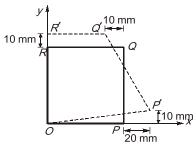
The horizontal displacement of the point (0.5 m, 0.5 m) in the plate O-P-Q-R (in mm, round off to one decimal place) is \_
